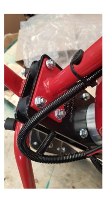
Unscrew right silenblock then fix the cable (blue connection)
