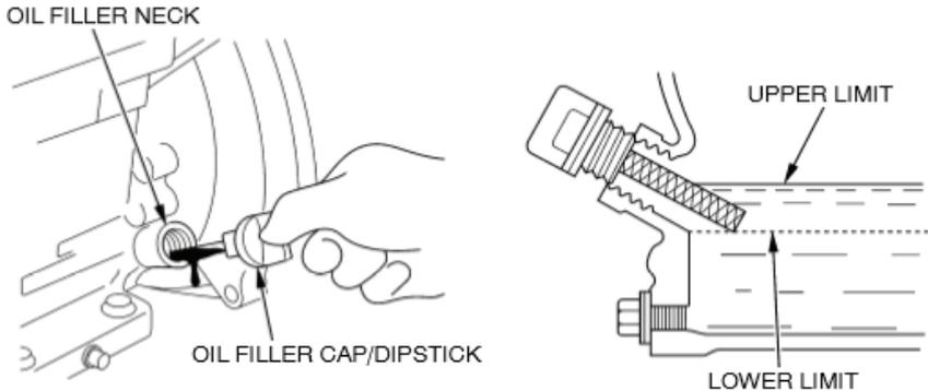
Running the engine with a low oil level can cause engine damage.
