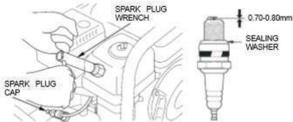
4. Measure the spark plug electrode gap with a suitable gauge. Correct the gap if necessary, by carefully bending the side electrode. The gap should be: 0.028 – 0.031 in (0.70 – 0.80 mm).
