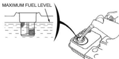
Do not fill above the shoulder of the fuel strainer (maximum fuel level).
